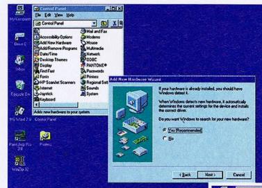
1. When you've installed your network cards and the cable, switch on your PC and Windows 95 should automatically pick up the new hardware. If for any reason it doesn't, select Add New Hardware from My Computer/Control Panel and let Windows automatically search for New Hardware.
