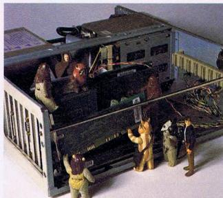
1. Switch both machines off and remove their cases, so you can see the expansion slots into which the expansion cards are plugged. These may be mounted vertically or horizontally, depending on the design of the PC. Find an empty slot in each machine and remove the blanking plate behind it by undoing the single screw at the top of the plate.
