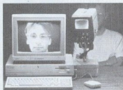
■ A typical digitising set-up, composed of an Amiga, a video camera, a digitiser and a lead.
