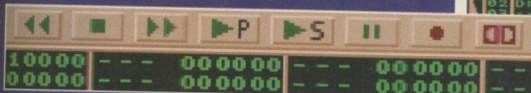
▲ The main controls are styled on the transport buttons of a tape recorder. The Dolby-style button toggles the lowpass filter.
