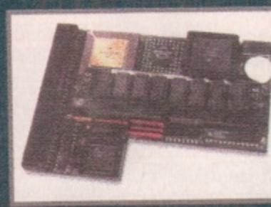
Accelerator card for the A1500/2000. Available in 25 & 50Mhz versions, complete with 68882 FPU & SCSI-2 interface. Not compatible with GVP cards.
