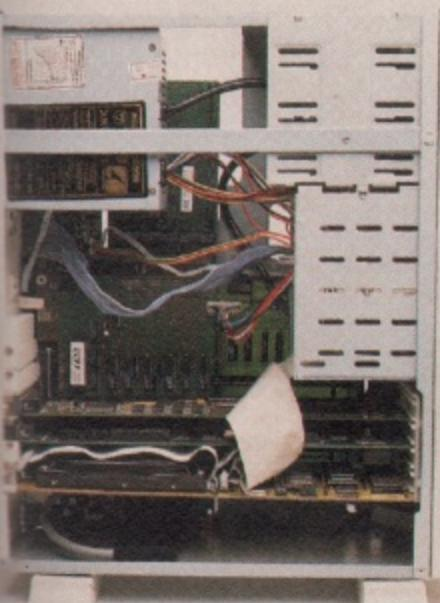
We have a fully loaded tower with the 230W power supply visible and a Squirrel SCSI at the bottom plugged into the PCMCIA right slot. In the middle there are three Zorro cards, GVP Spectrum card, GVP IO expander and an Octagon SCSI hard card. Rockin'!
