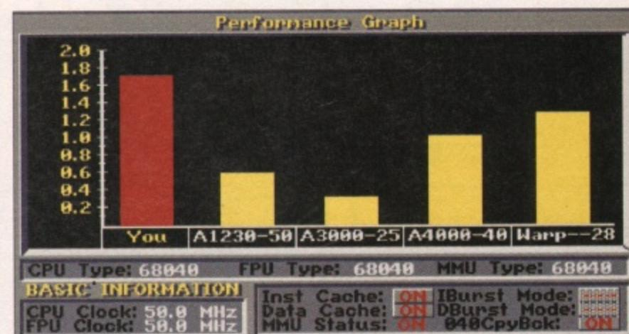
▲ The emulation test. Here the 50MHz 68040 shows what it's capable of on a good day while running typical emulator code such as PC-Task or Frodo.
