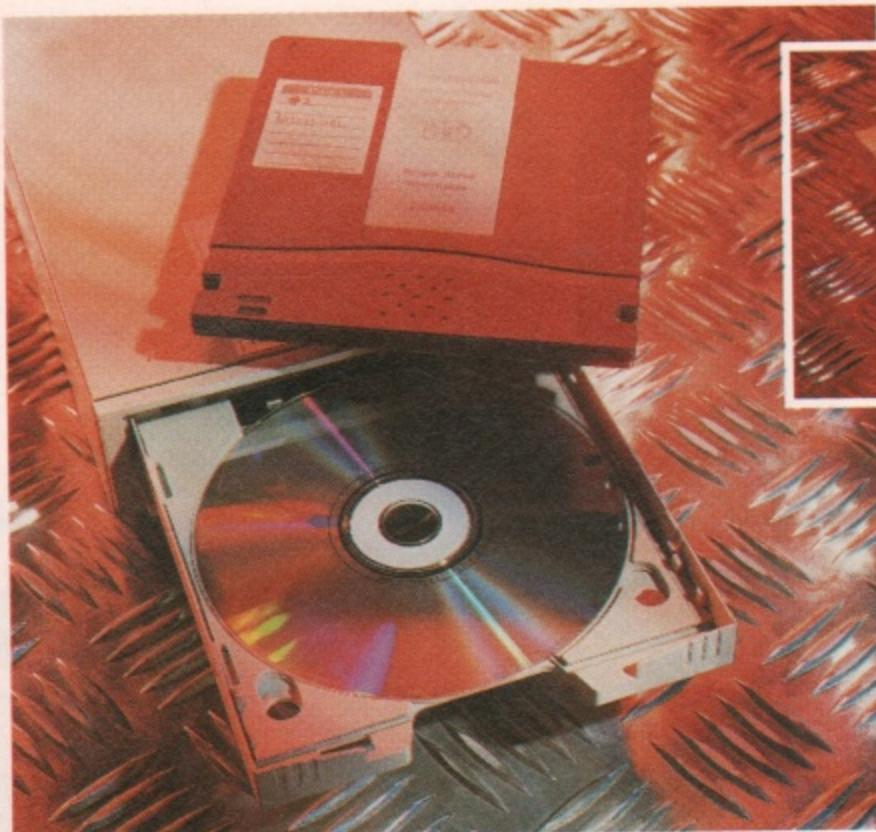
▲ The mighty MultiData machine. Seen here with a CD-ROM in place, the caddy also takes the 650Mb optical cartridge shown on top of the unit. The MultiData drive represented the lowest pence per megabyte cost.
