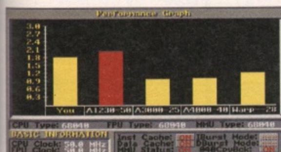
▲ The raytrace test using FPU co-processor code. The 50MHz 68882 is faster than the 68040 due to the missing instructions in the 68040.
