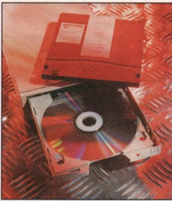
▲ The dual purpose platter of the MultiData machine takes either a CD as shown or a 650Mb optical cartridge shown on top of the unit.
