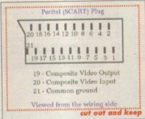
The SCART system packages all sorts of video and sound signals into one cable. Above: the essential connections you'll need to watch TV on a suitable monitor.
