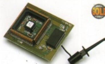
Increase your Amiga 500/2000 chip RAM to a total of 2MB. MegaChip does this by using its own 1MB of RAM and drawing extra memory from any other RAM you have installed in your Amiga. No soldering is required.
