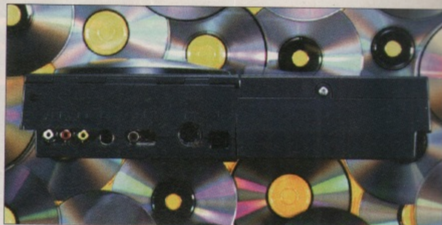
The rear view of the console shows the commitment Commodore have made towards making this a machine capable of supporting not only games, but Full Motion Video titles as well. Not only are there composite and modulated outputs, but also an S-Video port for S-VHS compatible images with better resolution than many of today's home videos.
