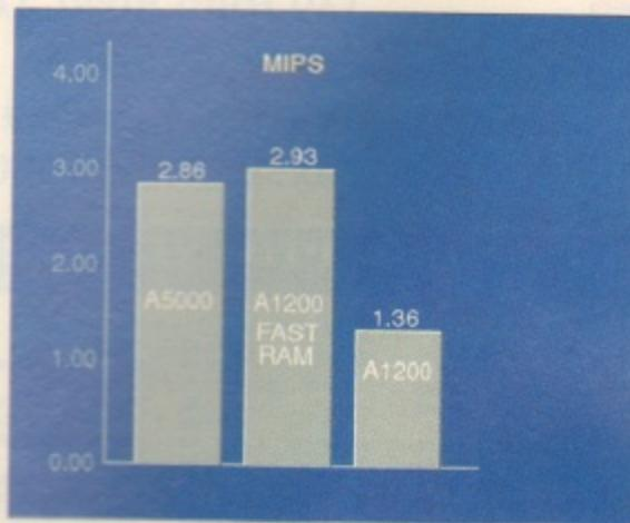
Using SysInfo V3.01, the relative speeds of the A5000 and A1200 (with and without fast RAM) were measured.
