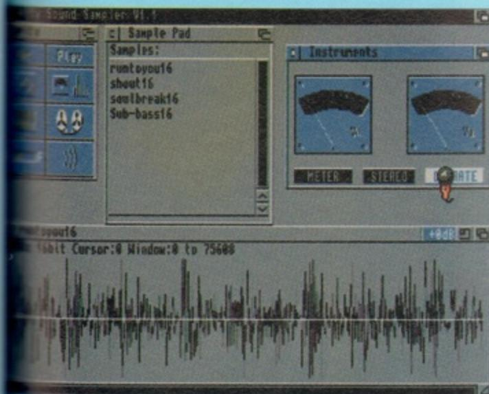
Monitoring your input before sampling can be done with any of the three scopes. The VU meters are prettiest, but the oscilloscope is probably the most useful.
