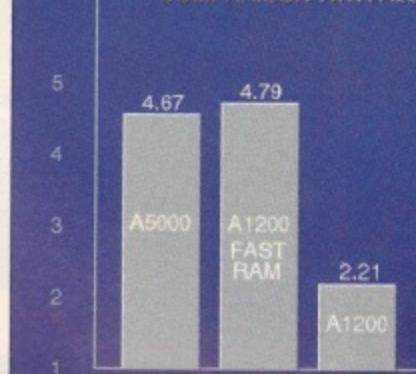
The graphs show how many times Sysinfo thinks the accelerated Amigas are faster than a standard 1Mb A5000. The Fast RAM makes a large difference to the A1200.
