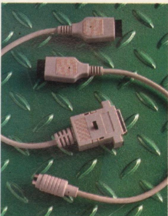
then connect the other end of the cable to your Amiga joystick port. A 3-way switch at the 15-pin end gives varying sensitivity levels. A neat little widget for anyone big on flight simulations. Digiprint also do a similar converter that allows you to use a PC mouse with the Amiga.
