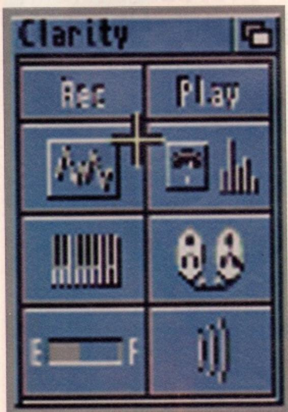
Most of the main sections of the Clarity software can be called up from this small control panel, which sits at the top left of the Workbench screen, although you can move this, and any other windows where ever you like.
