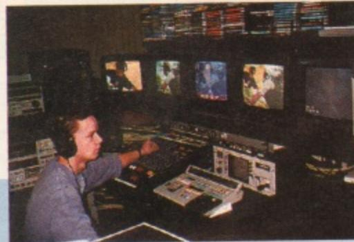
Sound is added via an 8-channel mixing desk. Note the DVE unit to the right.
