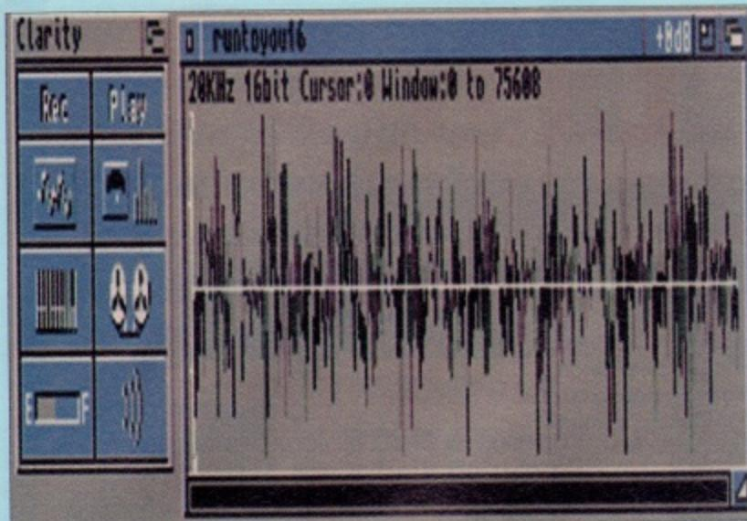
Here's one I prepared earlier. Each sample has its own editing window, which can be scaled, positioned, opened and closed as you wish.
