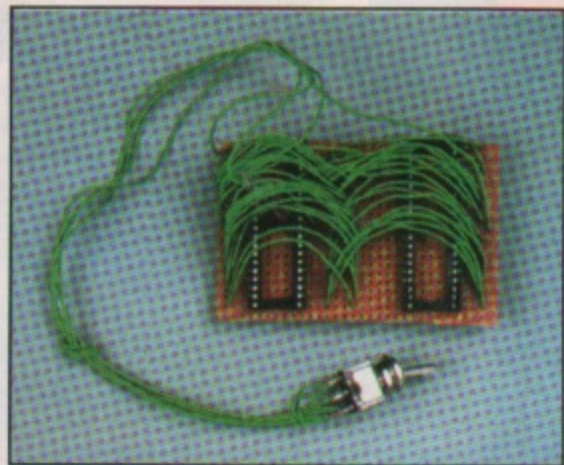
Be sure to use longer wires if you want to be able to get the ROMs in and out easily.
