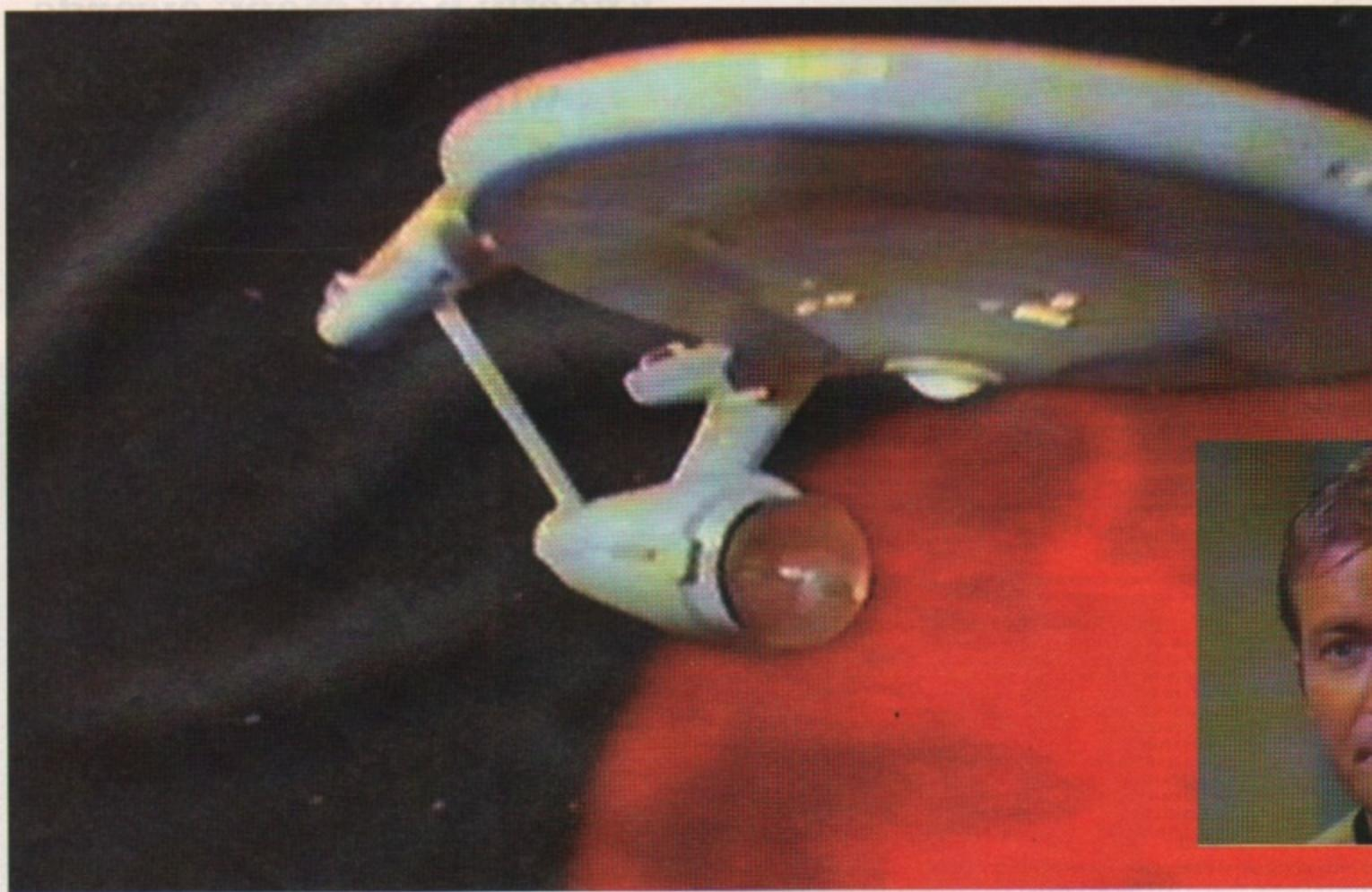
The colour bleeding in these pictures is not the fault of V-Lab, but of the PAL broadcast system and composite source.
