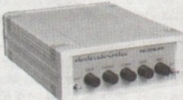
Built in high performance Phillips pal encoder enable perfect video fades. External colour, contrast and limminance controls allow total control to enhance video input. The built in RGB splitter allows digitised images to be grabbed from camera or recorder and fed through the genlock. Key inverter allows foreground and background to be switched in and out. Full superimposing with keyhole effect. PAL Genlock £349.99 Also available to support Hi-8, S-VHS £449.99
