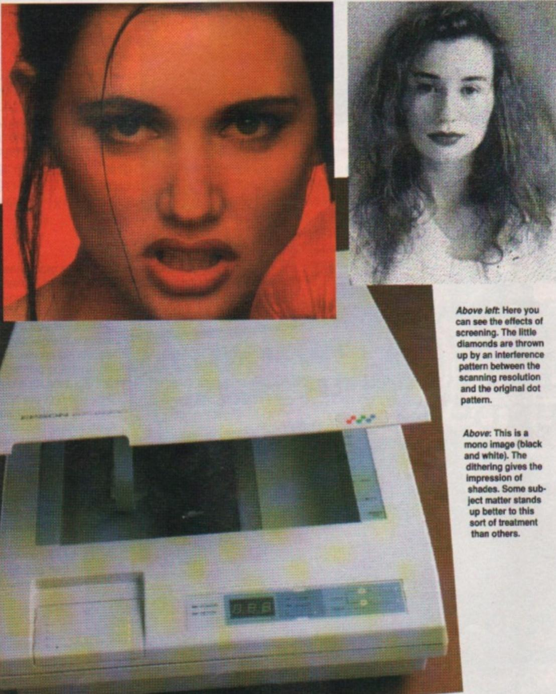
Above left: Here you can see the effects of screening. The little diamonds are thrown up by an interference pattern between the scanning resolution and the original dot pattern.
