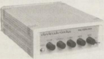
Built in high performance Phillips pal encoder enable perfect video fades. External colour, contrast and limminance controls allow total control to enhance video input. The built in RGB splitter allows digitised images to be grabbed from camera or recorder and fed through the genlock. Key inverter allows foreground and background to be switched in and out. Full superimposing with keyhole effect. **PAL Genlock £349.99** Also available to support Hi-8, S-VHS £449.99
