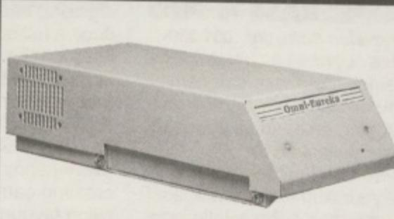
External 8MB ram expansion for Amiga A500. Full implemented auto configuring. Standard 1MB x 8 or 1MB x 9 simm modules. External power supply unit included. Memory test software included. Pass through bus design. High performance zero wait-states.
