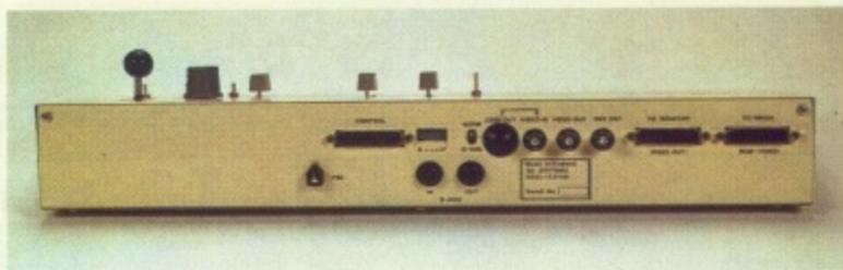
Above: The back of the box of tricks where the G2 VideoCenter Plus communicates with the Amiga and video recorder.
