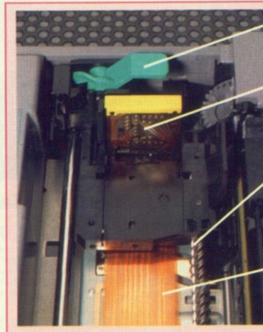
**Locking lever:** This secures the ink cartridge in place.
