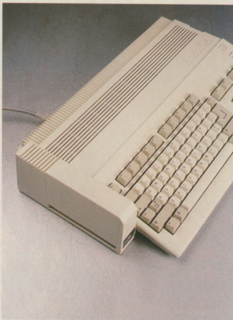
Video Digitizer II plugs into the extension slot at the side of the Amiga. It also includes a through-port which allows you to connect additional peripherals such as a Hard Drive.
