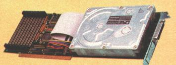
The HC8+ is a high speed hard drive & RAM card which can also be used to increase your Amiga's RAM by up to 8Mb.
