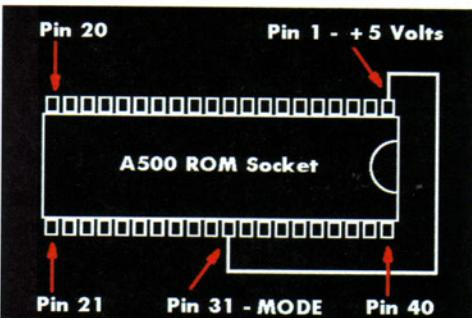
Here's how to do it - just solder one wire from pin 1 of the ROM socket (seen above from above) to pin 31.
