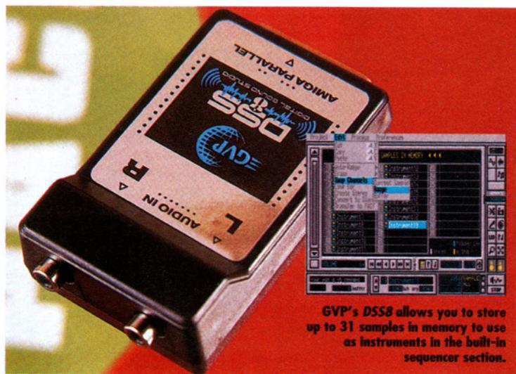
*GVP's DSS8 allows you to store up to 31 samples in memory to use as instruments in the built-in sequencer section.*
