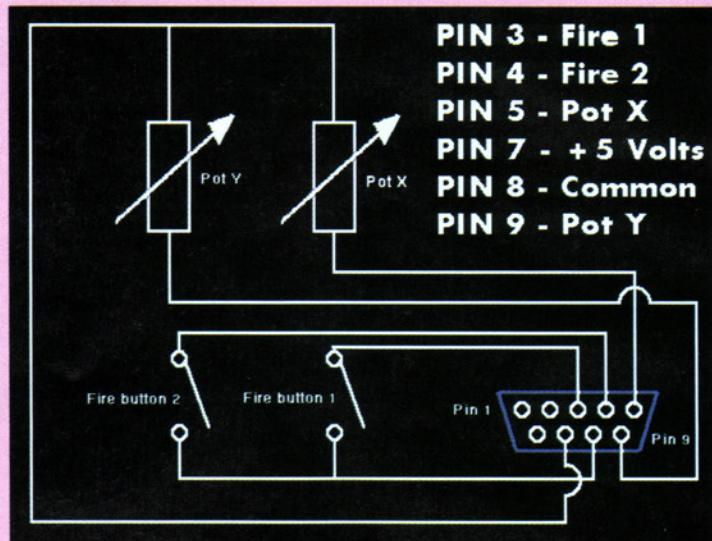
This is the official way to wire a proportional joystick on the Amiga. Some games assume the fire-button is on pin 6, rather than pins 3 and 4. Also, pin 1 can serve as a third fire-button. Be very careful what you do with pins 7 and 8. Pin 7 is the +5 Volt power supply, and pin 8 is the 0 Volts Ground or Common. Never the two shall meet or your Amiga will simply blow a fuse.
