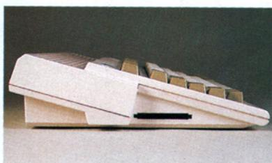
**The joystick ports are moved to the side of the Amiga, which is vastly more convenient. Note the wedge shape and the slanted disk drive.**
