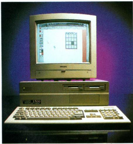
The A1500 is closely based on the A2000 (it shares the same motherboard) although some A1500s lack PC connectors on the inside.
