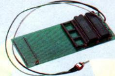
The Power Kickstart ROM Switch fits into any A500 or A500+ and can be fitted with up to three Kickstart ROM's and can be enabled when you switch on your Amiga.
