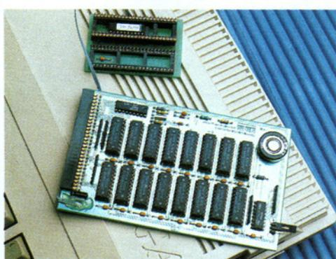
Trapdoor RAM boards, such as this one from Ashcom, are limited to the A500, and cannot be used on other Amigas.
