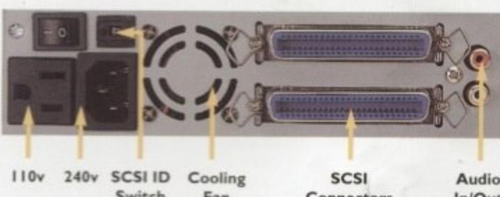
110v 240v SCSI ID Switch Cooling Fan SCSI Connectors Audio In/Out
