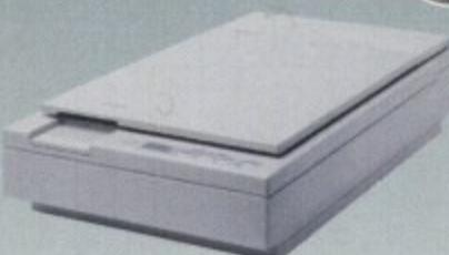
The Epson GT-6500 24-bit colour A4 flatbed scanner has output resolutions up to 1200DPI in 16.7 million colours, greyscale and line art. The GT-6500 comes with software, cables and manual.
