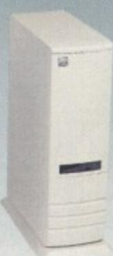
The A4000 Tower comes complete with 6 x 5.25" drive bays, 5 x 3.5" drive bays, real time clock, 7 x Zorro slots, 5 x PC slots and a 230 watt power supply unit.
