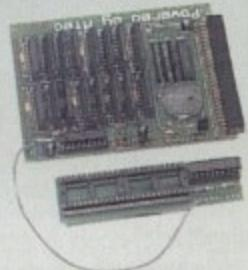
A 2MB RAM board for the A500 which fits in the trap door slot.
