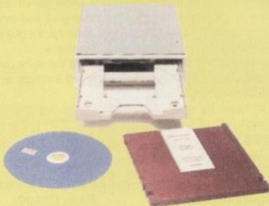
Well the wait is over and the future has arrived in the shape of the new Panasonic PD System Optical drive. This unit is a Hybrid 650Mb, Quad speed CD-ROM and Optical Read/Write system. (Yes, you did read that correct!). Now you can read all of your favourite CD Titles at over 600Kb per second and by inserting the low cost 650Mb cartridges you have 650Mb of storage space always on line just like a conventional hard drive.
