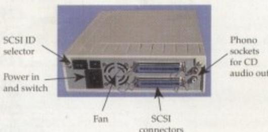
All our Squirrel Storage Systems come either bare (int - ready for installation internally within a suitably-equipped Amiga or other computer) or fully-cased (ext) with integral power supply, SCSI in/out, SCSI ID selector and audio out (for CD-ROM). The cases we supply are high quality, shielded, snap-together enclosures, each with 40W power supply - the back panel of the 5.25" case is shown above. These SCSI enclosures are available at £69.95 each (please specify 3.5" or 5.25" when ordering).
