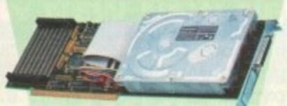
The HC8+ is a high speed hard drive and RAM card which can also be used to increase your Amiga's RAM by up to 8Mb RAM.
