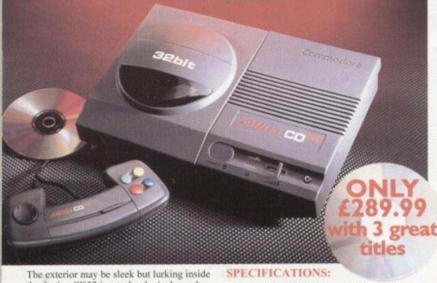
The exterior may be sleek but lurking inside the Amiga CD32 is a technological wonder. At its heart is the mighty powerful 68EC020 processor from Motorola. This contains the 32-bit technology which has made the Amiga 1200 a runaway success throughout Europe.
