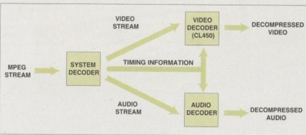
*This is how a basic Mpeg decoder system links up*
