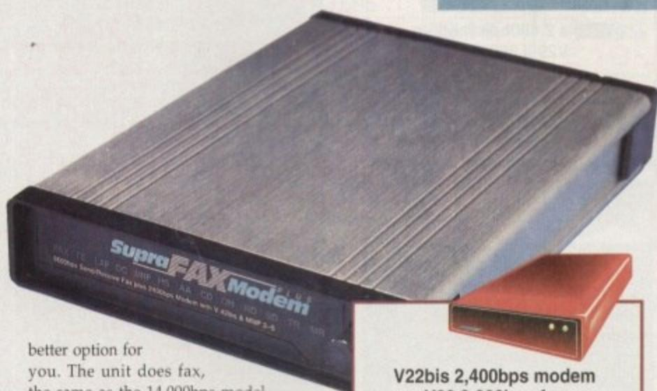
better option for you. The unit does fax, the same as the 14,000bps model, but at 9,600bps, and does data at 2,400bps. So it's basically a bog standard 2,400 modem with MNP, not unlike my old machine, but it has the fax added on, hence the name.
