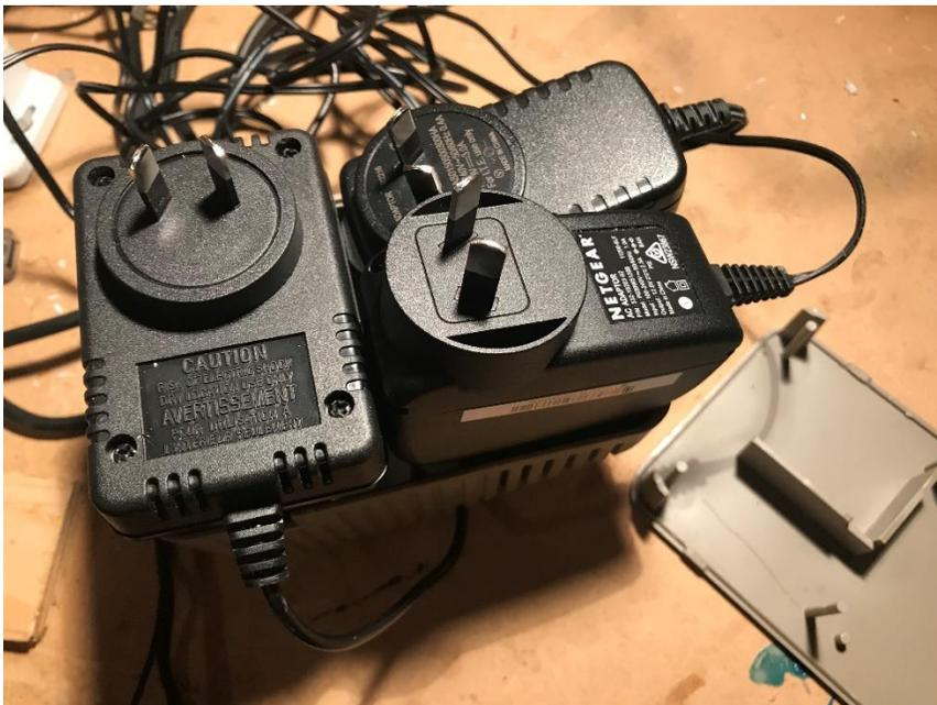
Wow, there is more room in the old brick than I thought. This gave me an idea. What if I could fit the contents of 3 power packs into this one brick. I obviously needed the 9V AC and 5V DC, but I found an old router power supply that delivered 12V DC. I've always wanted to see if I could have a small 12V
