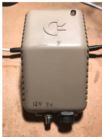
I then realized that not only could this power supply power a C64 and a 12v monitor, it could also power any floppy drives that needs 12v and 5v DC. So, I then obtained the connector used on my 1581 drive.
