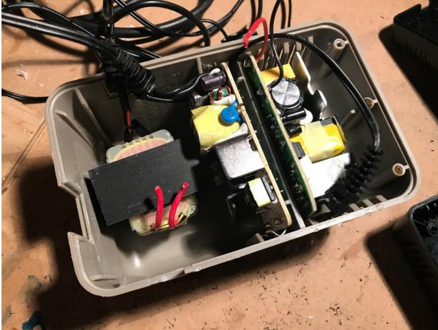
Next, I placed each of the 3 power supplies into the empty brick. The transformer that delivers 9V AC is shown here on the far-left hand side at the bottom (which becomes the top when the brick is turned back over to be the right way up), the middle one is the 12V DC power supply, and one on the right is the 5V DC power supply.
