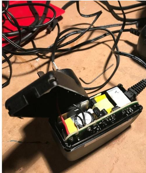
Here is the Netgear power pack that was able to break open (a couple of screws and a bit of firm but careful prizing with a flat blade screwdriver) and get out the 12V DC power supply from within.
