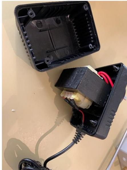
I did the same with the 5V DC power supply and the 9V AC power pack (the 9V AC was the easiest as it just had 4 screws to remove and it opened).
