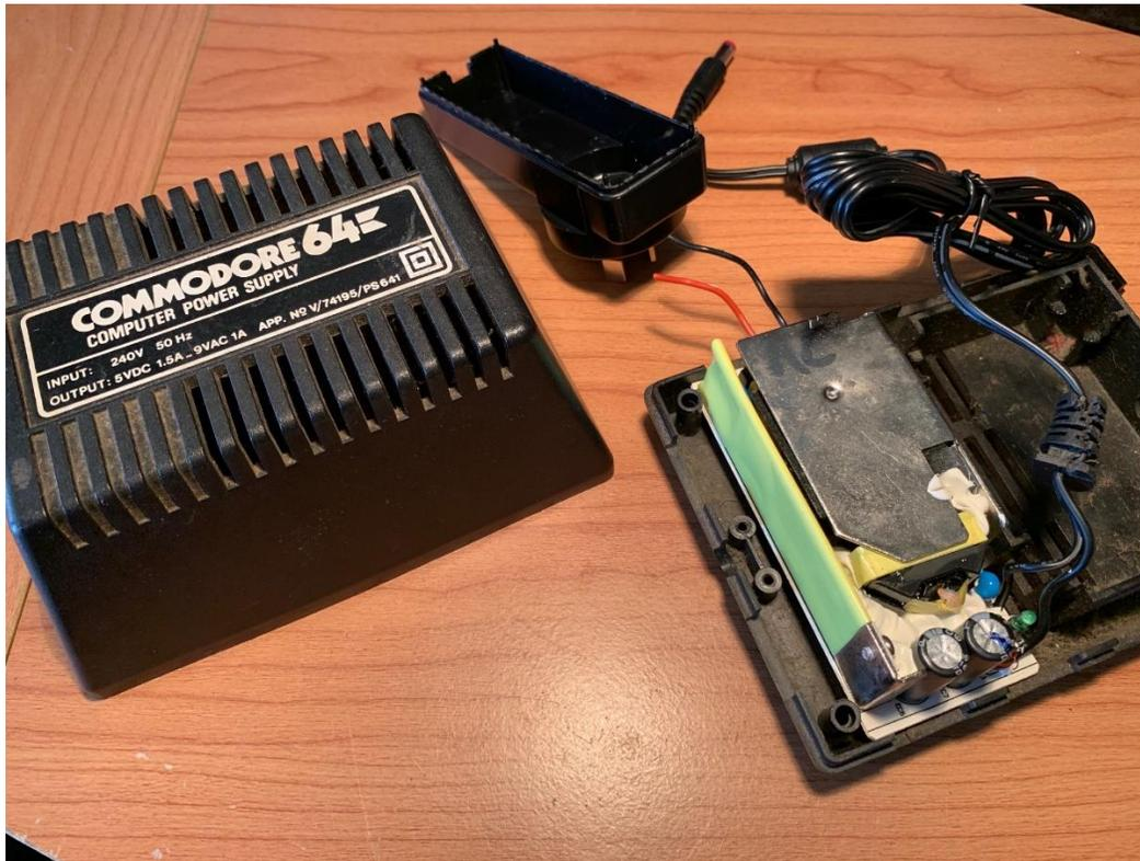
These types are much easier to work on, as there are just 4 screws to undo to open the unit and once the old transformer and rectifier are removed above, you can see there is heaps of room to put some supplies rescued from un-used power adapters. Here I've installed the 12v supply from a router I don't use anymore.
