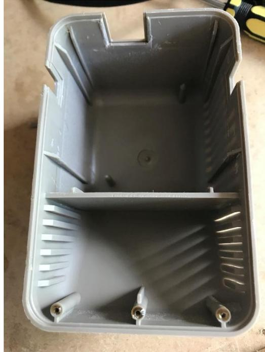
After cutting away the old wires, I found that with some flexing of the sides and hitting the unit, right side up, down onto my workbench, that the inside started to slide out. Here I am using a pair of pliers to pull the old power supply out leaving an empty shell. Apparently, the old transformers are very reliable and could be re-used, but I couldn't be bothered trying to
