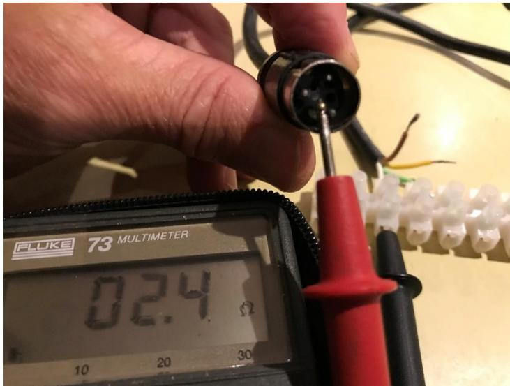
Here I am testing the white wire to confirm it does indeed go to pin 5 using a multi-meter.
