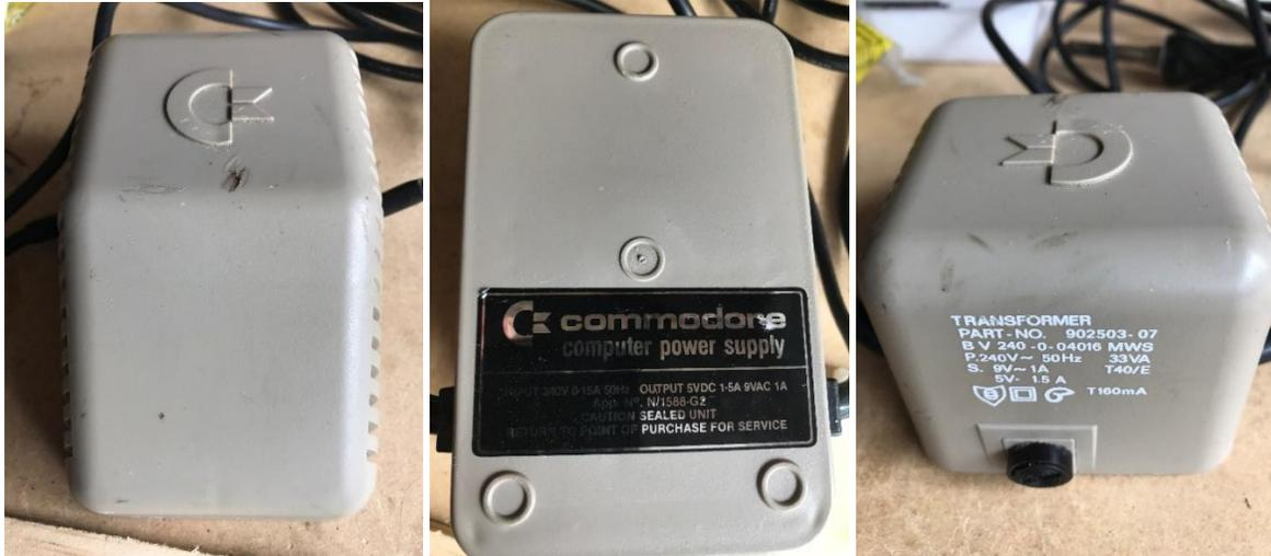
For this project I decided to take an old Commodore 64 power supply and 're-brick' it by first emptying it of the current contents (as these are old and the 5V DC can often fail, going high and potentially damaging your Commodore 64), and filling the inside with new modern components as taken from standard power packs.
