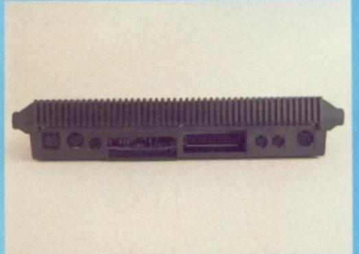
*The plus 4 matches the 64's interfaces. The reset button is the only addition.*
