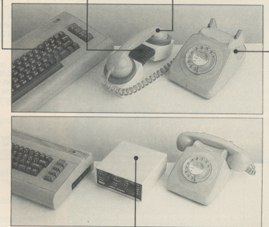
The telephone plugs into the modem, and the modem plugs into the telephone socket.
