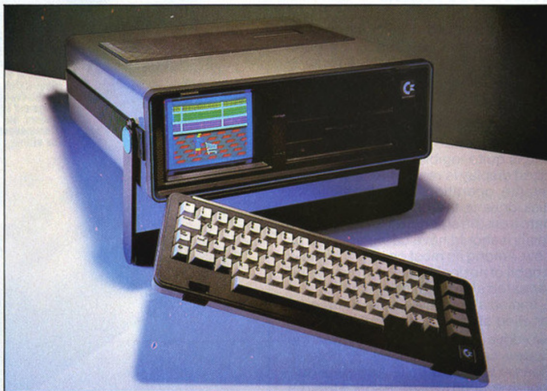
The SX-64 uses the carrying handle to act as a rigid stand when the machine is being used desktop-style.
