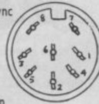
Pins 1 and 6 provide the 'Commodore Video' output for the 1701 monitor, while Pin 4 provides the 'composite video' output for non-Commodore monitors.
