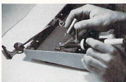
After re-soldering the shift-lock key wires, reverse the procedure for reassembly.
