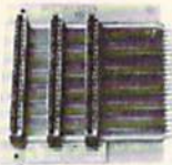
Slot for the VIC. No switches, reset, or fuse.
