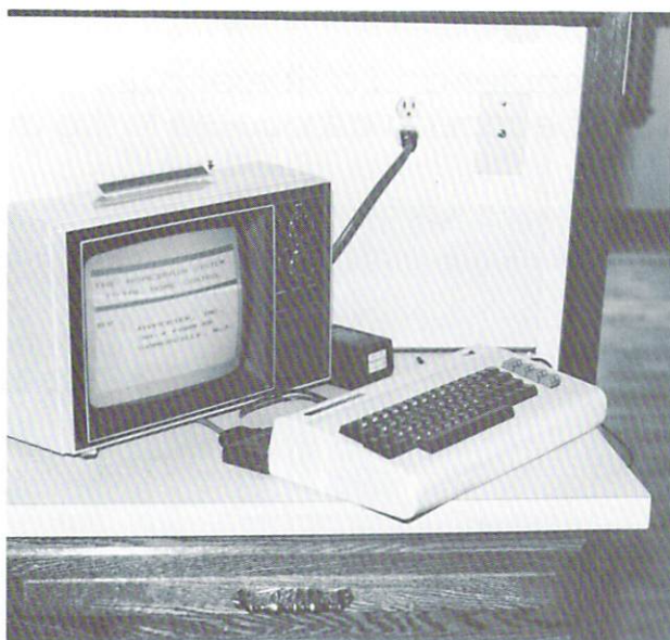
In the kitchen of the model home, the VIC 20 and monitor can be hooked up to communicate with the Homebrain in the basement.
