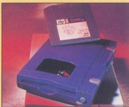
The Zip from Iomega is a removable cartridge system that is fast increasing in popularity. It has an almost magical ability to fit just under 100Mb of data onto cartridges that are only marginally bigger than floppies. Could this be the end of the floppy as we know it?
