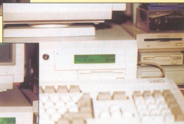
Above: The completed Liquid Crystal Display (LCD) in place in my A4000.
