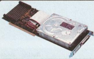
The Impact II HC8 hard cards are the equivalent of the HD8+ hard drive, but for the 1500 and 2000 models. They are some of the fastest hard drives available, and incorporate an unpopulated 8MB RAM expansion.
