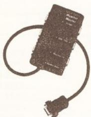
This monitor switch box for the vortex Golden Gate automatically identifies when PC or Amiga graphics should be displayed.
