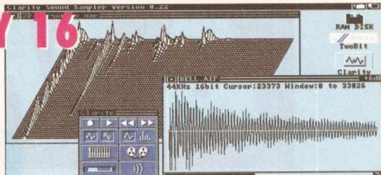
**Clarity 16** produces incredible CD quality sound on your Amiga. Microdeal's hardware/software package enables you to sample and play back sounds at an incredible 16-bit resolution. Frequencies of up to 44.1KHz can be sampled. Full editing facilities, including special effects, are provided with *Clarity 16*'s software.
