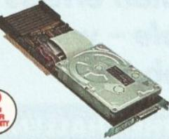
The Impact II HC8 hard cards are the equivalent of the HD8+ hard drive, but for the 1500 and 2000 models. They are some of the fastest hard drives available, and incorporate an unpopulated 8Mb RAM expansion.
