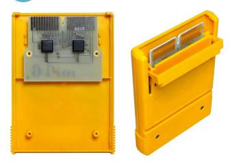
Fig. 4 - The inside of a Videocart and the contact protection flap (photo: Schnurrikowski- source: Wikimedia Commons)
