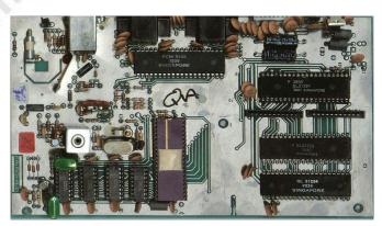
Fig. 2 - The motherboard of the Channel F System II. Note the few integrated circuits present (photo: Incog88 - source: Wikimedia Commons)
