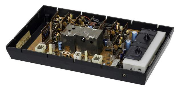
Fig. 4 - Interior of the Odyssey. You can see the circuits made with discrete components (photo: Evan-Amons)
