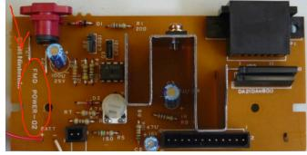
FMD-PWER-OX where instead of the X there can be a number between 1 and 5; revision 1 is unprotected, revision 2 may have it sometimes not, revision 3 is probably unprotected while revision 4 and 5 definitely implement protection.
