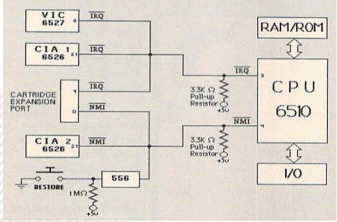
Fig. 1 - Sources of Hardware Interrupt Requests to the 6510 CPU in the Commodore 64
