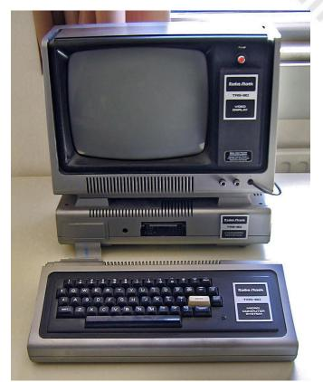
Fig.4 - A TRS-80 Level I (note the keyboard without the numeric keypad) with Expansion Interface (the additional case placed under the monitor) (photo by Flominator, source Wikimedia Commons)
