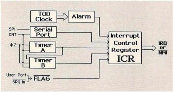
Fig. 2 - Detail of possible Sources of the 2 CIA chips
