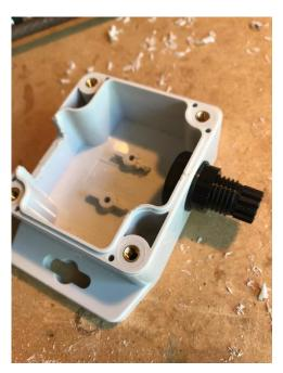
On the opposite side I drilled a hole large enough to mount a cable gland (again from JayCar), to hold the 2 cables that come from the 2 power packs.
