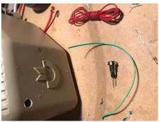
the legs. I then soldered 2 wires (red on the + side and green on the – side), and simply ran the wires to the 5V pins in the terminal block shown earlier.
