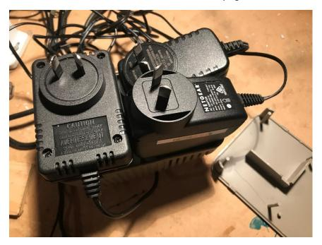
Wow, there is more room in the old brick than I though. This gave me an idea. What if I could fit the contents of 3 power packs into this one brick. I obviously needed the 9V AC and 5V DC, but I found an old router power supply that delivered 12V DC. I've always wanted to see if I could have a small 12V
