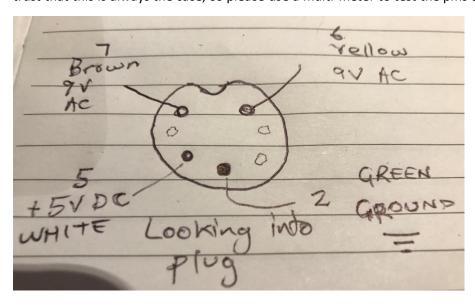
Pins are looking into the front of the plug (i.e. mirror of the back of the plug or looking at the C64).
