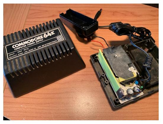
These types are much easier to work on, as there are just 4 screws to undo to open the unit and once the old transformer and rectifier are removed above, you can see there is heaps of room to put some supplies rescued from un-used power adapters. Here I've installed the 12v supply from a router I don't use anymore.
