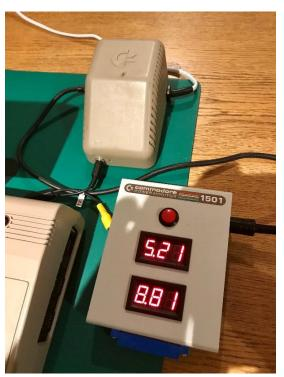
A quick check to ensure the voltages are right on the pins of the Commodore 64 power cable.
