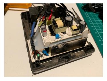
Here I decided to just mount the 5v supply (this was another that I also got from a power adapter) right on top of the 12v. I put a layer of plastic (just cut a rectangle out of the side of a milk bottle) as insulation between the 2 supplies.
