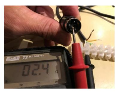
Here I am testing the white wire to confirm it does indeed go to pin 5 using a multi-meter.
