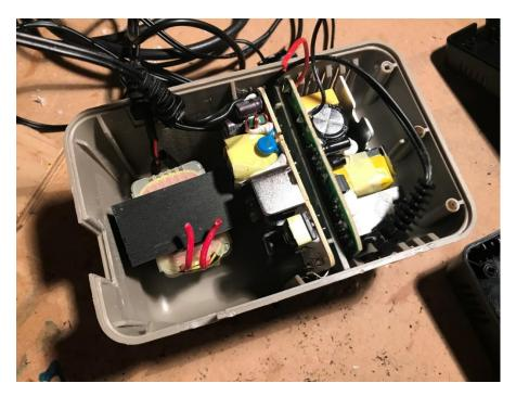
Next, I placed each of the 3 power supplies into the empty brick. The transformer that delivers 9V AC is shown here on the far-left hand side at the bottom (which becomes the top when the brick is turned back over to be the right way up), the middle one is the 12V DC power supply, and one on the right is the 5V DC power supply.
