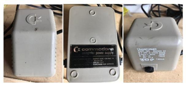
For this project I decided to take an old Commodore 64 power supply and 're-brick' it by first emptying it of the current contents (as these are old and the 5V DC can often fail, going high and potentially damaging your Commodore 64), and filling the inside with new modern components as taken from standard power packs.
