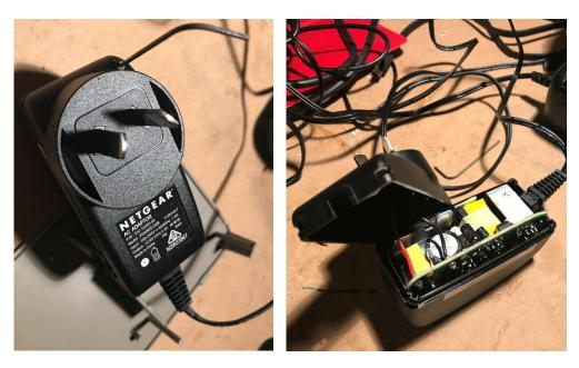
Here is the Netgear power pack that was able to break open (a couple of screws and a bit of firm but careful prizing with a flat blade screwdriver) and get out the 12V DC power supply from within.
