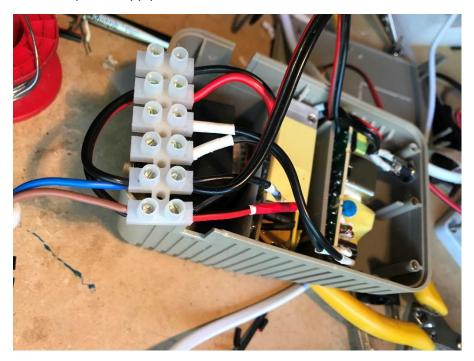
I then soldered new wires as needed to the 3 power supplies and terminated them onto a 6 wide terminal block. This allowed me to have the 240V AC mains power come in (shown on the bottom 2 terminals being the blue and brown wires), then the 5V DC and 9V AC. I wired the 12V directly to a suitable female cabinet mount connector (as shown on the right hand side of the brick case).
