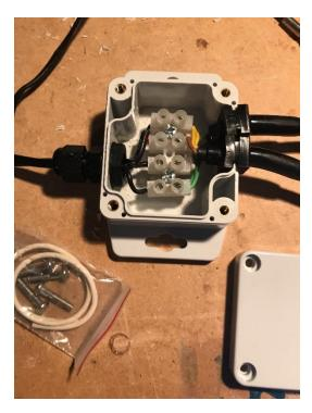
You may notice that I wired 2 Commodore 64 power cables on the right side of the terminal block, just so I could either power 2 C64s, or to show the power via a power monitor as you will see in the next picture. The 1501 Power Monitor is available online (eBay) from a fellow Australian maker.
