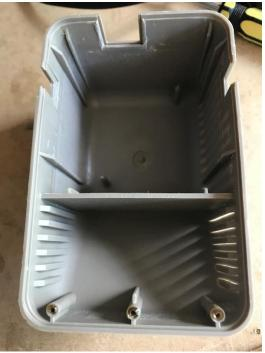
After cutting away the old wires, I found that with some flexing of the sides and hitting the unit, right side up, down onto my workbench, that the inside started to slide out. Here I am using a pair of plyers to pull the old power supply out leaving an empty shell. Apparently, the old transformers are very reliable and could be re-used, but I couldn't be bothered trying to
