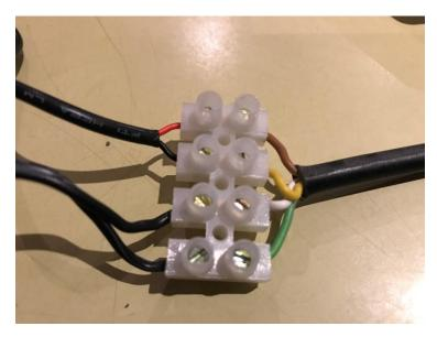
These terminal blocks are also available at JayCar or any similar outlet (or online). The top pair of wires is the 9V AC wires, and the bottom pair is the 5V DC. The top wires can be done either way around (AC voltage has no polarity to worry about), but you do have to make sure the DC is wired the right way around.
